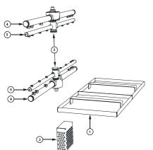
Remove scrap trays<sup>①</sup> and wash pump inlet filter<sup>②</sup>, where fitted, and rinse or brush clean.
