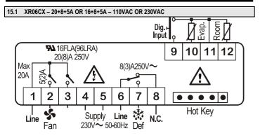
$\textbf{NOTE:} \ \text{The compressor relay is 20(8)A or 16(6)A depending on the model}.$
