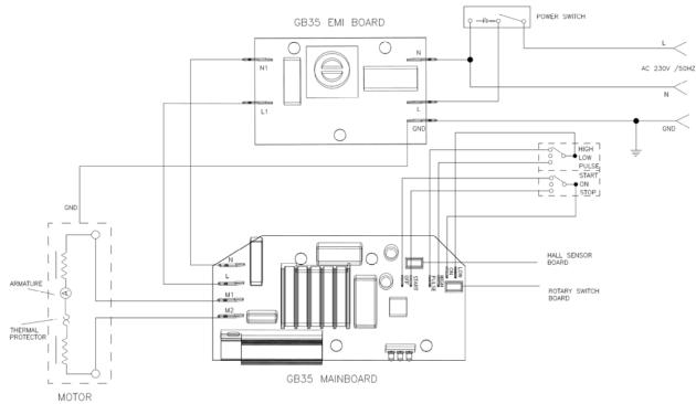
GB35 SCHEMATIC WIRING DIAGRAM
